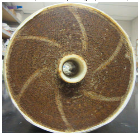
Figure 1: A scaled RO element. Photo courtesy of DHP Inc. (Farmington, New Mexico).
