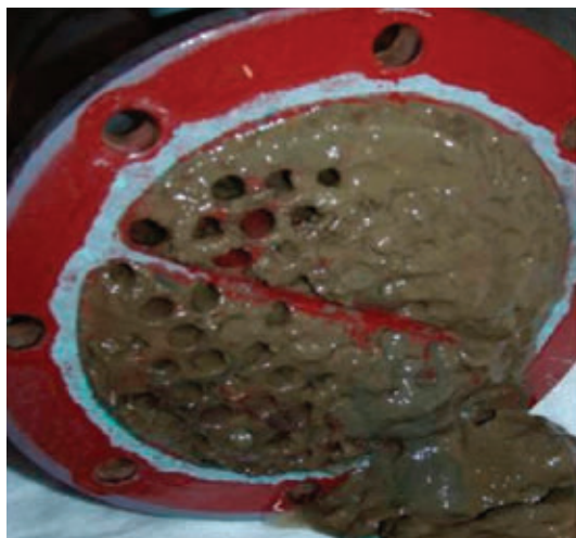
Figure 1: A heat exchanger fouled with microbiological slime and silt.
